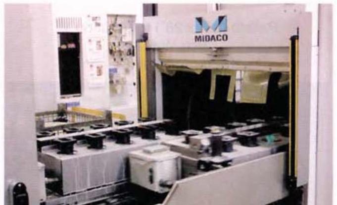
The fixtures shuttle in and out of the machine. The fixture going in is loaded with parts ready to be machined. The fixture coming out is full of finished parts.
