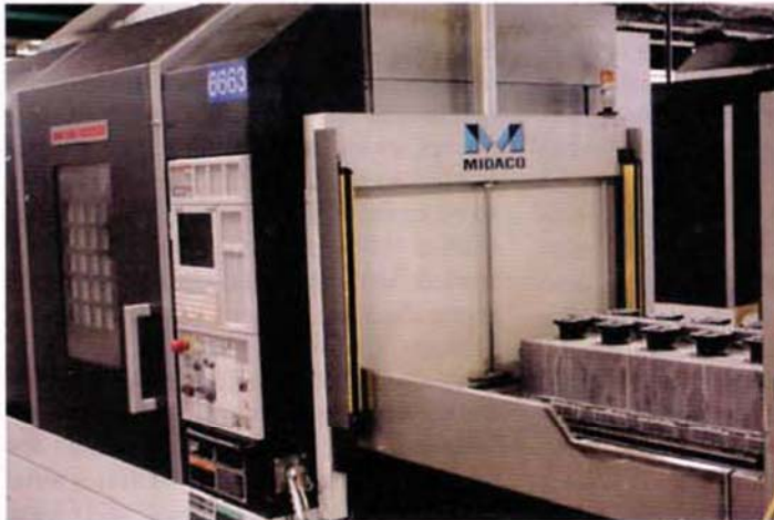
Fixture queued up ready to be transferred into the Mori Seiki DV5100 VMC machine by the Midaco automatic pallet changer.
