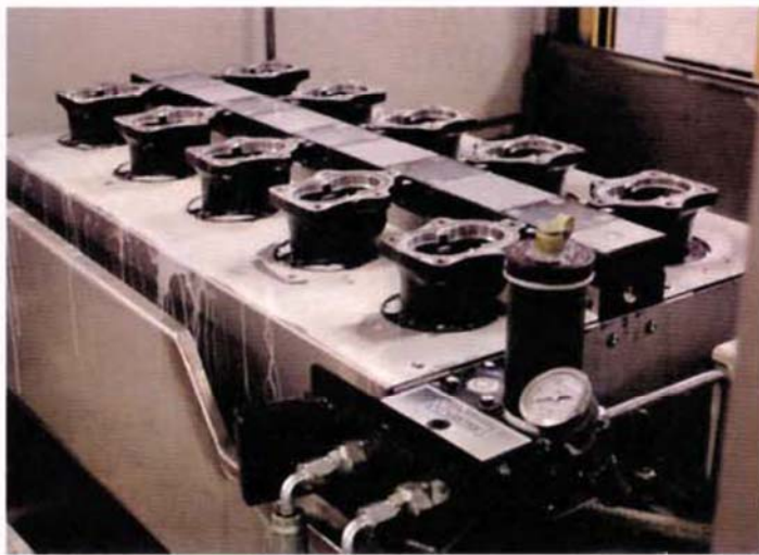
All ten parts loaded into the chucks on the fixture prior to being clamped. The external pressure system is coupled to the fixture to actuate the collets.
