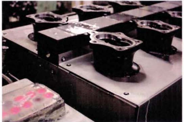
The LED system shows that eight of the 10 parts are seated correctly. The parts sit on three proximity switches in the workstop.
